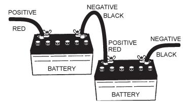
Figure 40. Battery Connections
